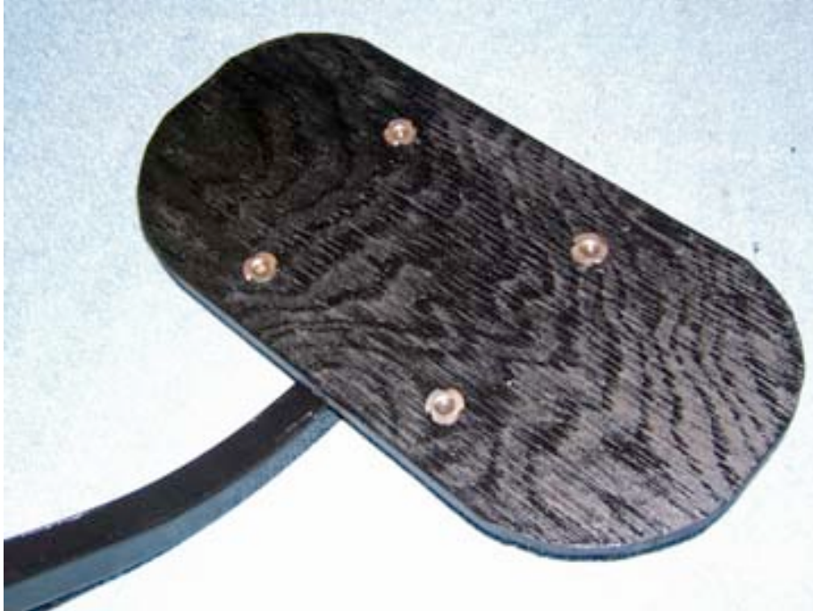
Tee-Nuts are visible. The visco-elastic foam was glued to the surface facing up in the picture using purpose-made aerosol glue.
